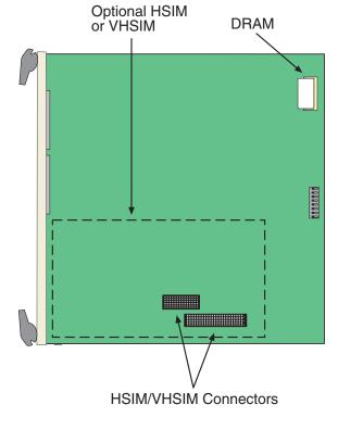
Figure B-4 HSIM and VHSIM Connector Locations
